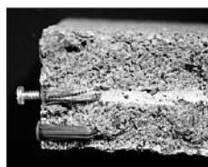
Plug anchor - NO extrusion & NO bonding
