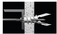
Tighten screw flush with item. The screw pops open the anchor, locking it on the wall and holding the gypsum board in compression. This reinforces the wall, increasing its holding power significantly.
