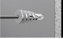
Press tip of SnapSkru anchor into drywall using PZ2 or Phillips #2 screwdriver or screw gun. Drive the anchor clockwise into drywall until anchor stops flush with the outer wall surface.
