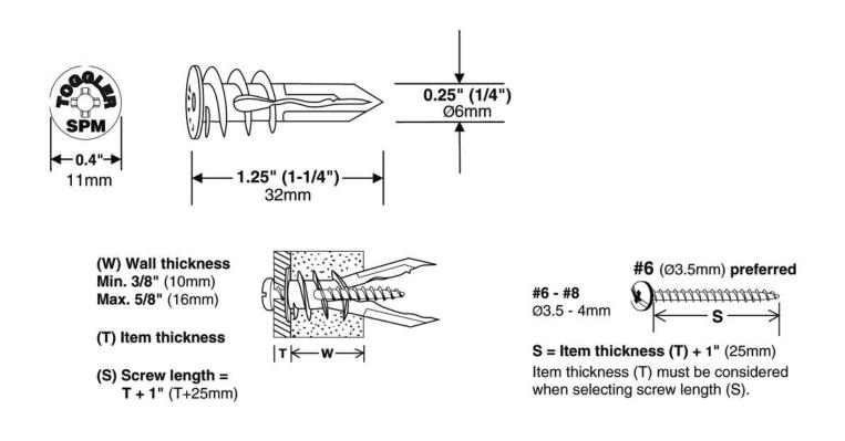
Description — SnapSkru MINI [SPM] Self-drilling Drywall Anchor
